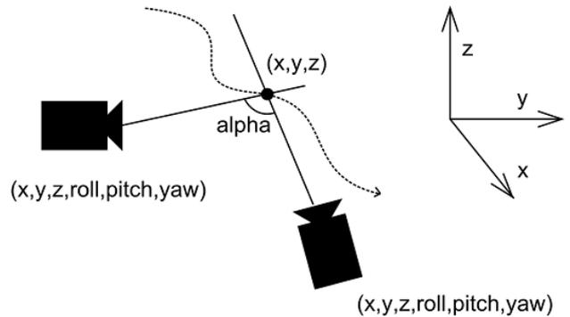
The first step in this process is to find the position and orientation of each camera used. This can be accomplished either as an off-line measurement assuming that cameras are not moved between calibration and actual test, or on-line, dynamically for each image allowing shaking/moving cameras.
